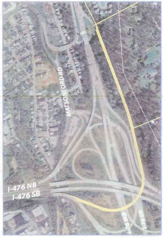
Concept of the relocated Conshohocken Interchange ramps along Matsonford Road. (Drawing prepared for DVRPC by the Louis Berger Group, Inc., 2008)
