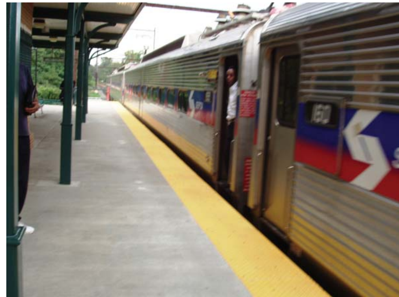
View showing high level platform at the same height as the floor of the rail car.
